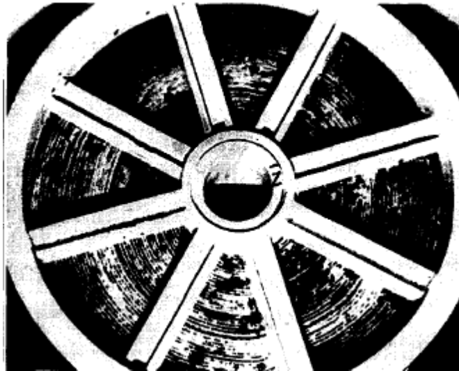
Figure 31: Biofouled spiral-wound membrane [23]
