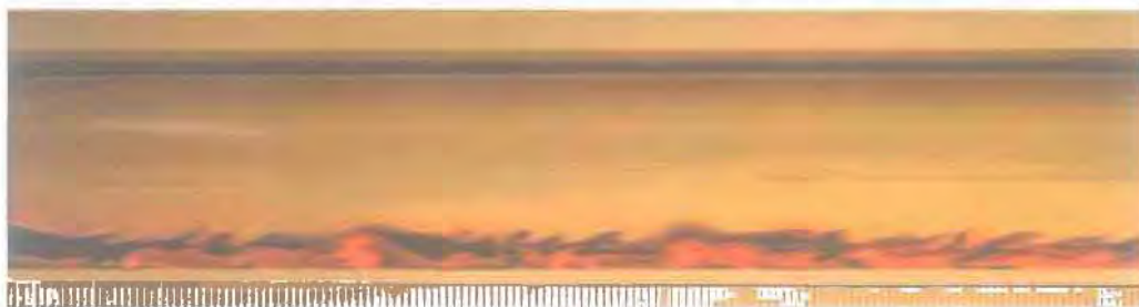
(γ) U_{LS}=0,008 m/s και U_{GS}=13,92 m/s κύματα Kelvin – Helmholtz
