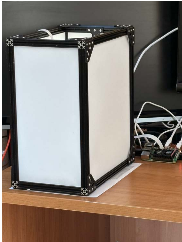
Figure 4.1: CubeSat-like incubator with mounted Raspberry Pi and camera
