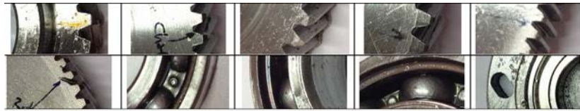
Figure 2.5: Faulty bearings and gears (source: [3]).
