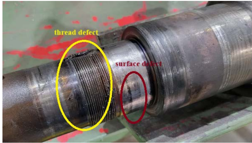
Figure 2.4: Possible defects of shafts.
