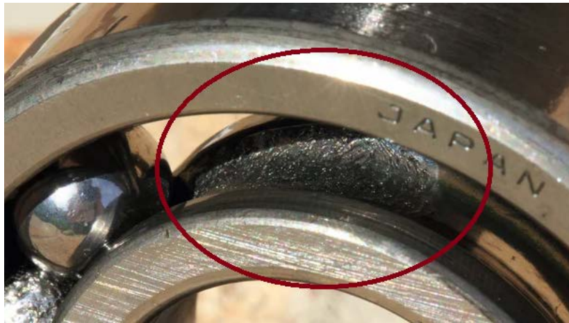
Figure 2.3: A bearing's defective outer raceway.
