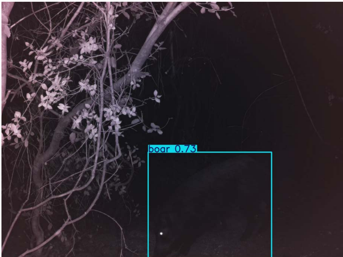
Figure 5.5: Boar Detection Example
