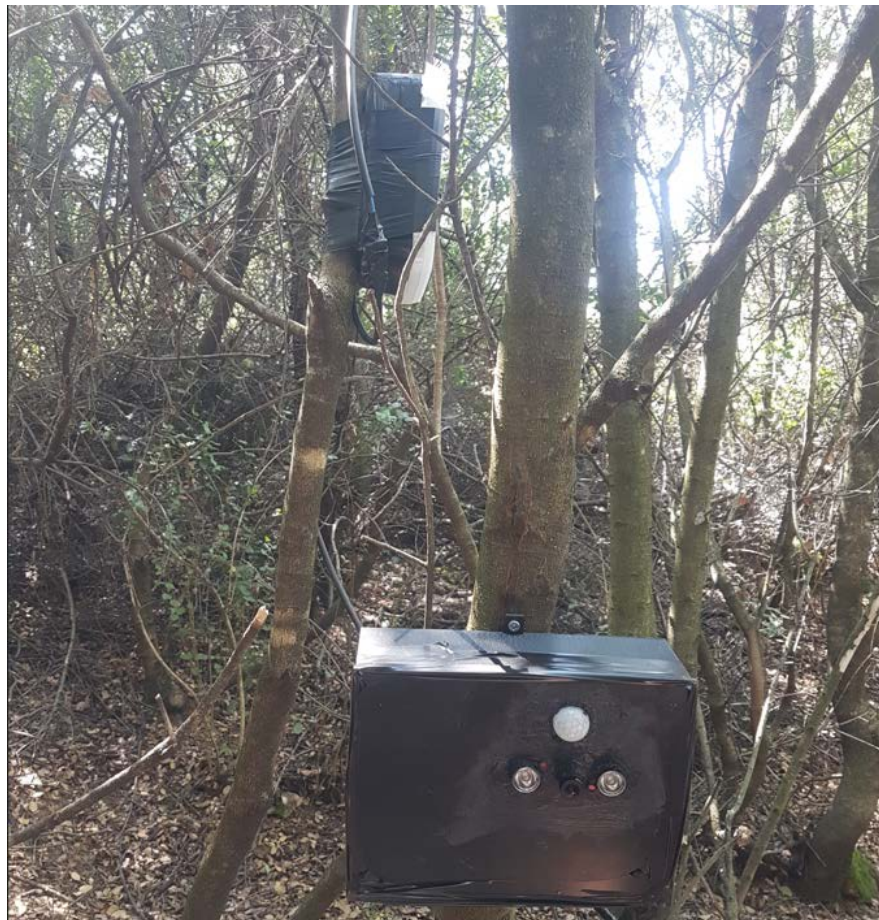
Figure 5.2: Device And Solar Power Manager
