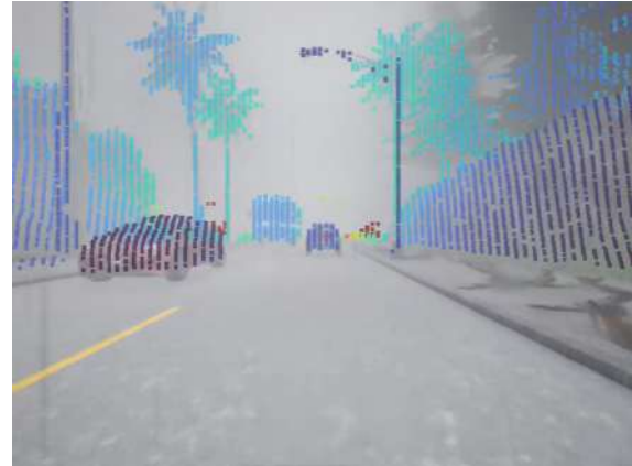
Figure 6.8: Depth-encoded 2D representation of LiDAR points.
