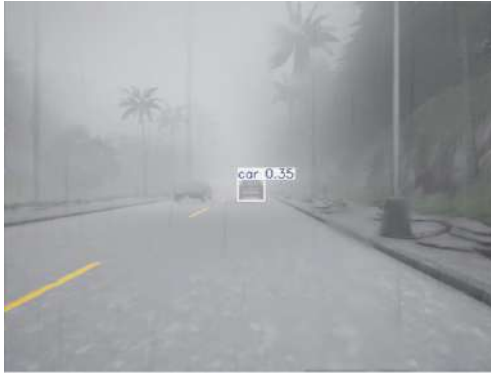
( \alpha' ) Example of YOLOv8 detection on a traffic scene in CARLA in bad weather.
