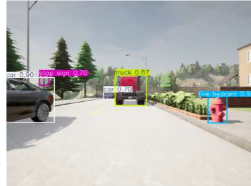
( \beta' ) Example of YOLOv8 detection on a traffic scene in CARLA in nice weather.
