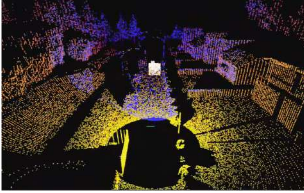
( \alpha' ) Radar points mapped and projected into the LiDAR frame.
