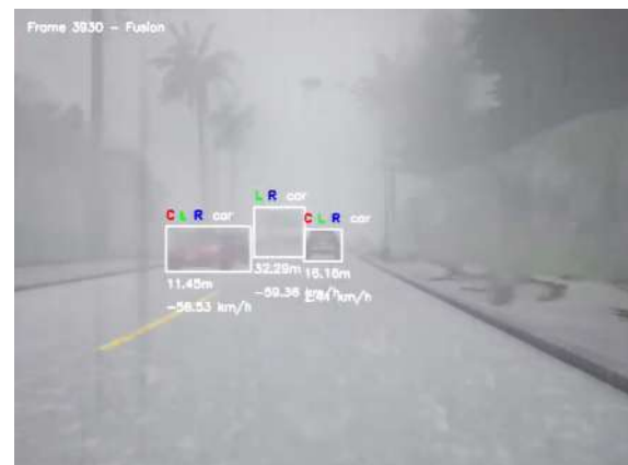
Figure 7.4: Result of early fusion: fused detection combining 2D detection.
