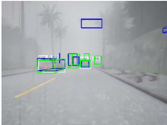
Figure 7.10: LiDAR, radar, and stereo detections into a common 2D image plane.
