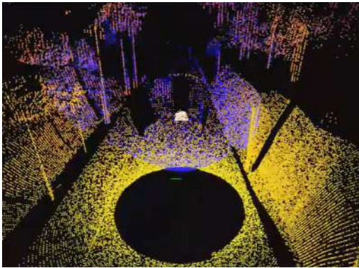
Figure 7.6: LiDAR and radar points merged into a common 3D point cloud.
