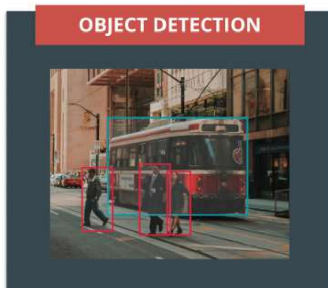
Figure 3.1: Detection Example in the 2D space
