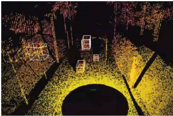
( \alpha' ) 3D Clustering of Lidar points
