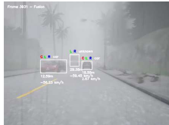
Figure 7.11: Visual result of late fusion detection in 2d plane.
