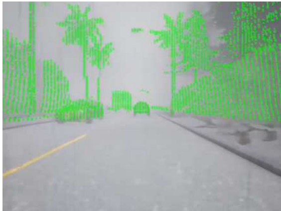
Figure 6.7: Non depth-encoded 2D representation of LiDAR points.
