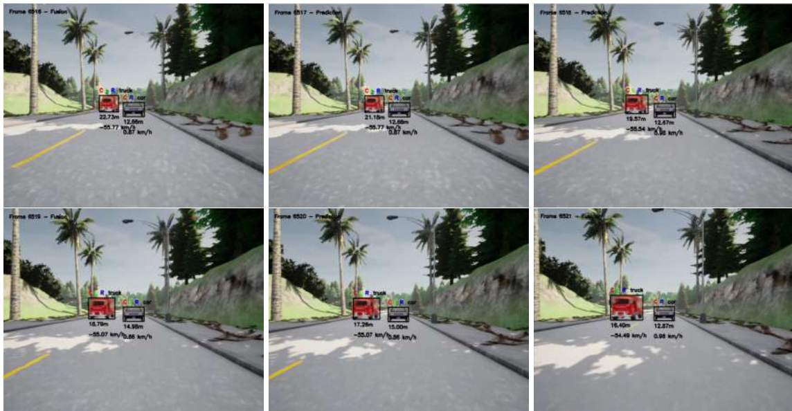
Figure 8.4: Example of multi object tracking. The temporal evolution of object positions is shown in the 6 frames.
