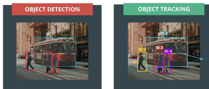
Figure 2.5: Object detection vs Object tracking [8]
