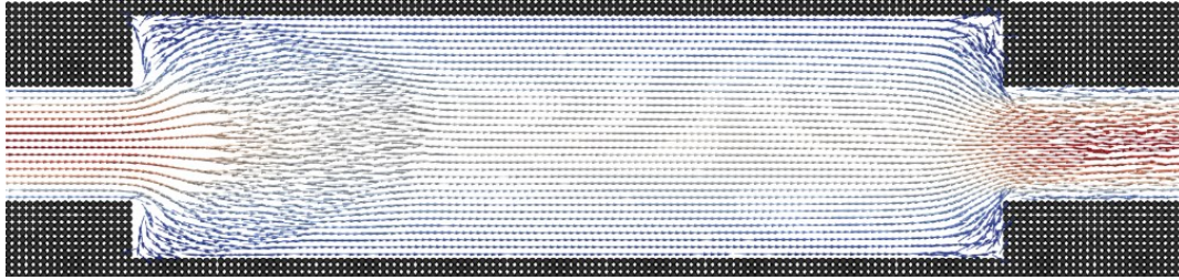
Figure 25. Two-dimensional sudden expansion/contraction. Trajectory lines (not to scaled) in the expanded section of the channel at t = 30 s.
