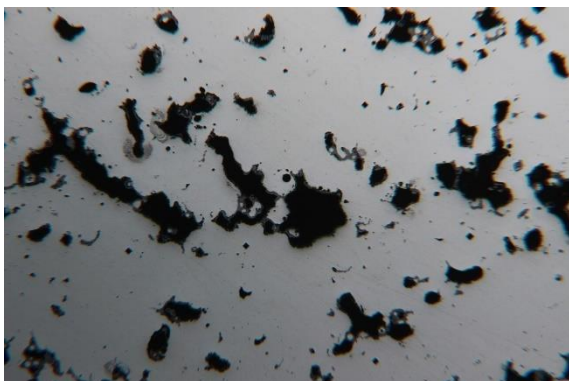
Figure 3.1 Original microscopic image of a specimen showing visible porosity ( \times 50 )
