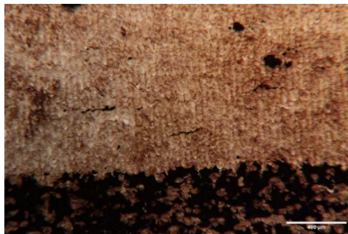
Figure 4.10: Three cracks at the center of as-built 1 (x50)
