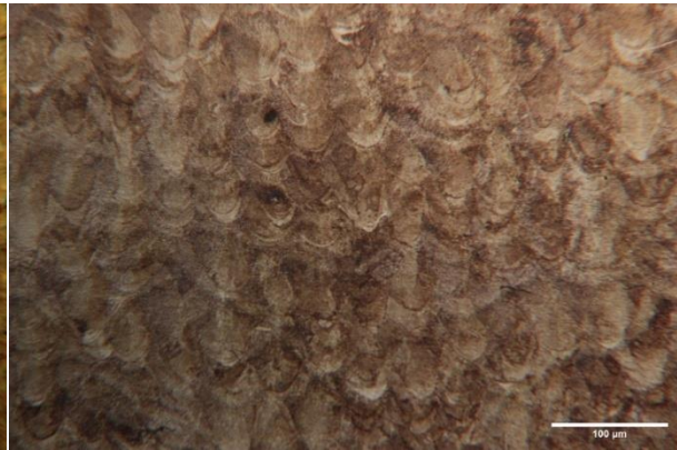
Figure 4.3: Microscopic transverse section at the center of as-built 1 (x200)
