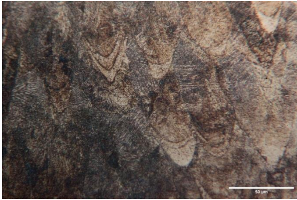
Figure 4.6: Melt pools at the top left (x500)
