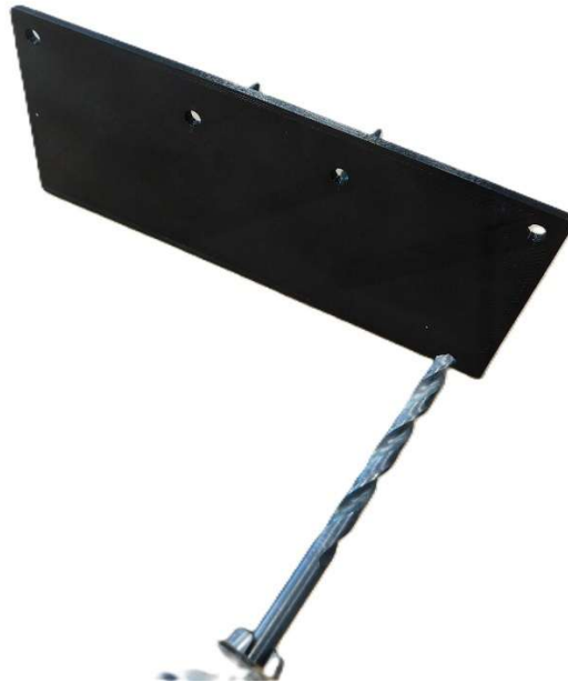
Figure 3.15. Cleanup with the use of a 3.8mm drill bit
