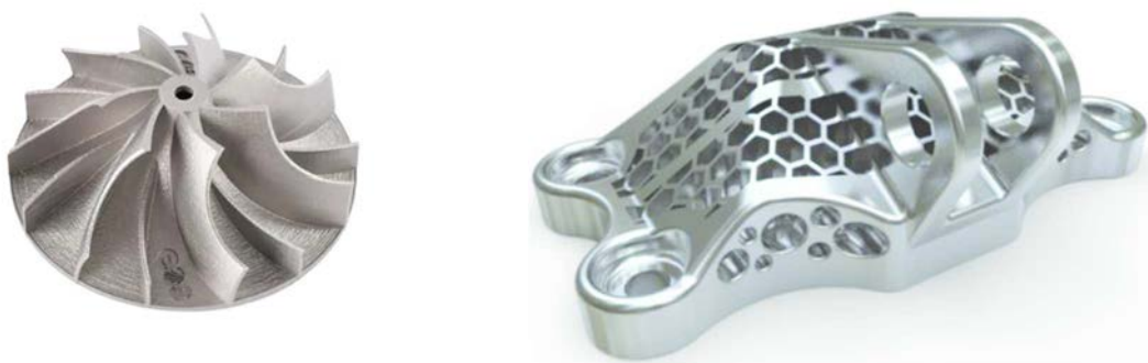
Figure 2.15. Example of parts manufactured through the DMLS method
