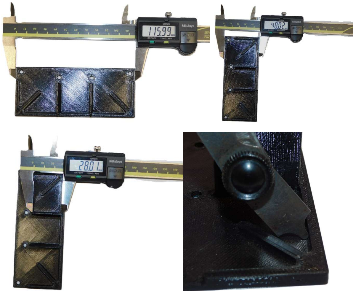
Figure 3.20. Basic measurements with caliper of FFF manufactured component
