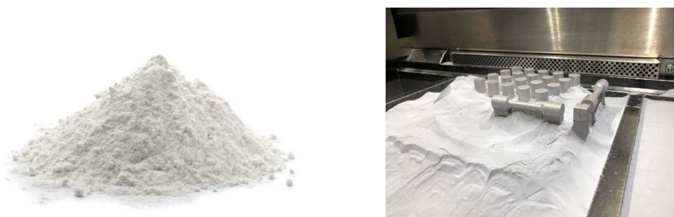
Figure 2.8. Example of the powder material used in the manufacturing process and manufactured parts in the machine after cooling
