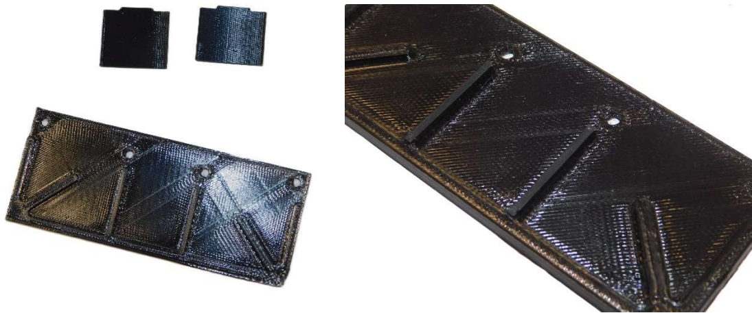
Figure 3.16. Layer delamination on perpendicular features
