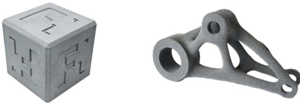
Figure 2.18. Example of parts manufactured through the MJF method
