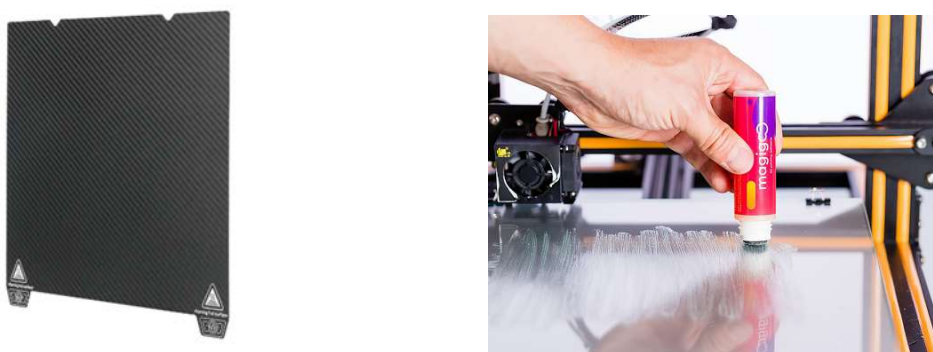
Figure 2.26. PEI build surface and glass build surface with the use of glue
