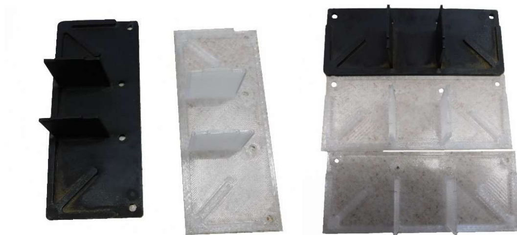
Figure 3.12. FFF manufactured parts with the original part
