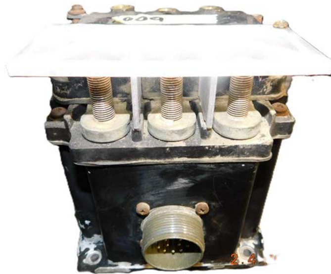
Figure 3.13. FFF manufactured part on the relay
