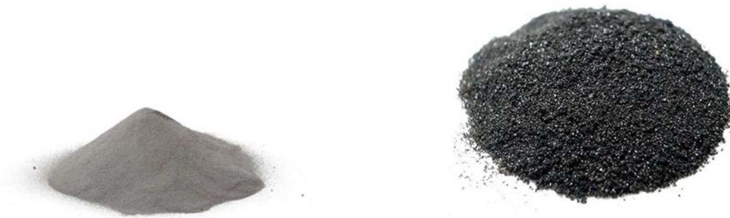
Figure 2.13. Example of the powder material used in the manufacturing process (titanium and AISI 1060)
