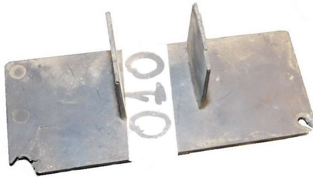
Figure 3.7. Original failed relay terminal cover
