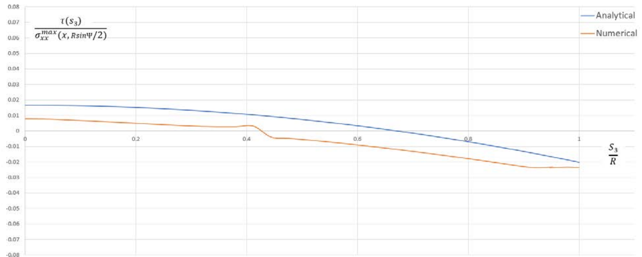
Figure 2.11: A-shell; normalized distribution of \tau \equiv \tau(s_3) across the length of the lower side CO of the aerofoil. The numerical solution is compared to the analytical.
