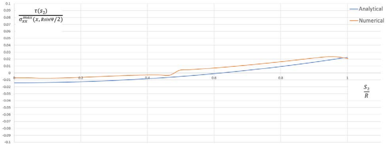
Figure 2.10: A-shell; normalized distribution of \tau \equiv \tau(s_2) across the length of the upper side AO of the aerofoil. The numerical solution is compared to the analytical.
