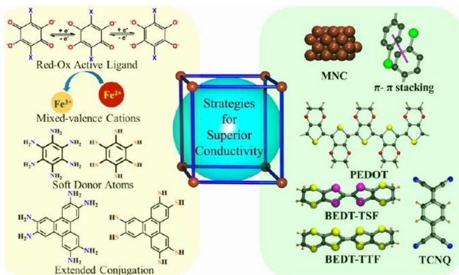
Figure 37: Schematic representation of intrinsic and extrinsic strategies for enhancing the electrical conductivity of MOFs. The left side highlights molecular-level design approaches, including redox-active ligands, mixed-valence cations, and soft donor atoms. The right side illustrates extrinsic methods such as \pi - \pi stacking, conducting guest molecules, and incorporation of metal nanoclusters. Color code: C = gray, S = yellow, Se = pink, N = blue, O = red, Cl = green [78].
