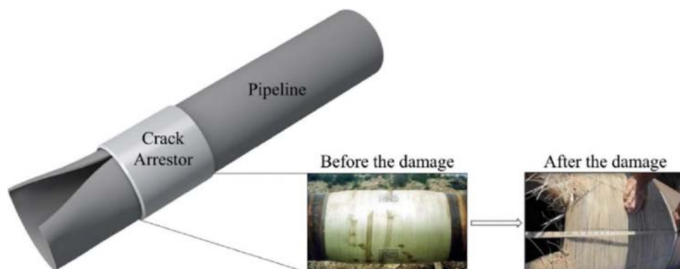
Figure 3.12 Crack arrestor on a pipe, before and after the damage [10]
