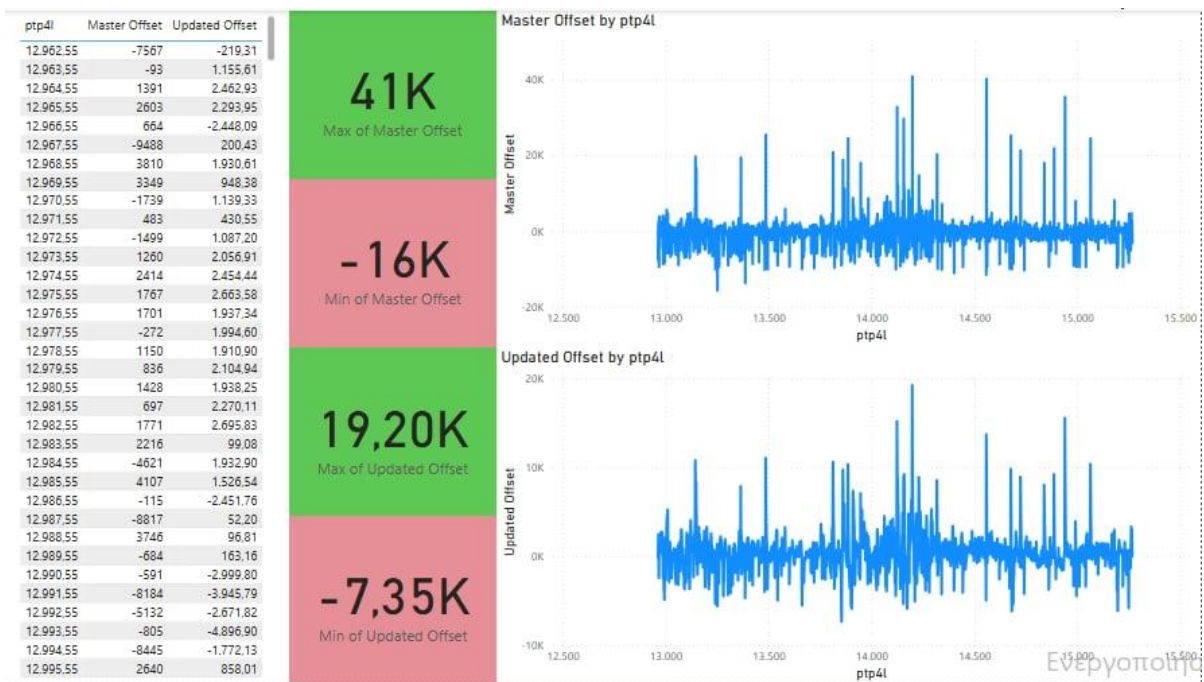
Figure 6 Offset Behavior During High Container Activity
