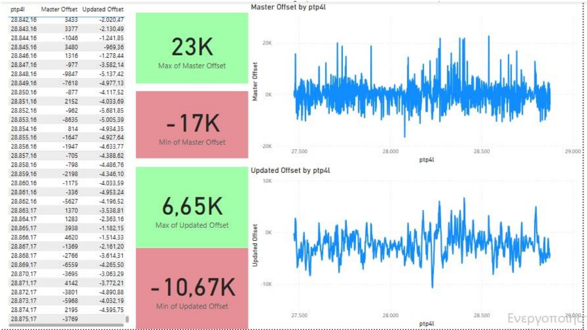
Figure 5 Comparison of Raw and Filtered Offset: Mid-Load Scenario
