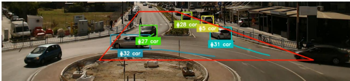
Figure 26: Polygon detection zone for spatial filtering of vehicle detections
