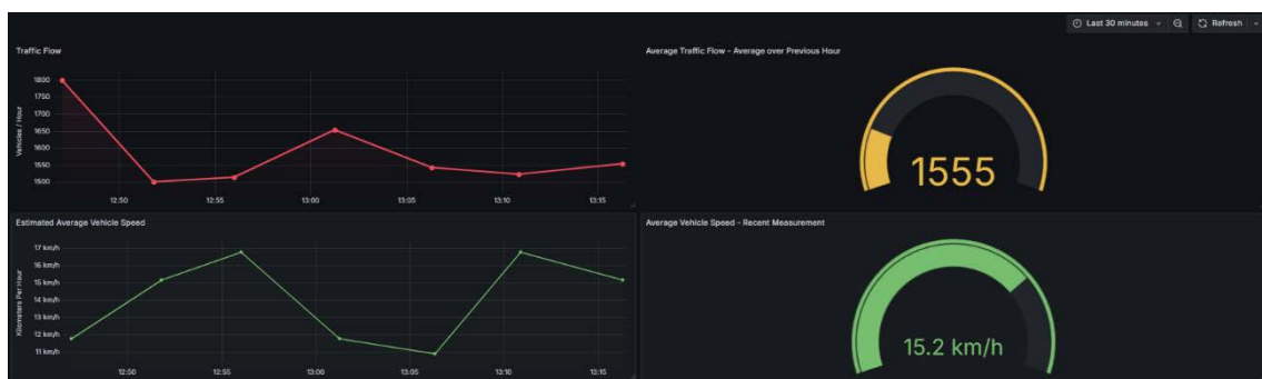
Figure 34: Traffic monitoring system's Grafana dashboard
