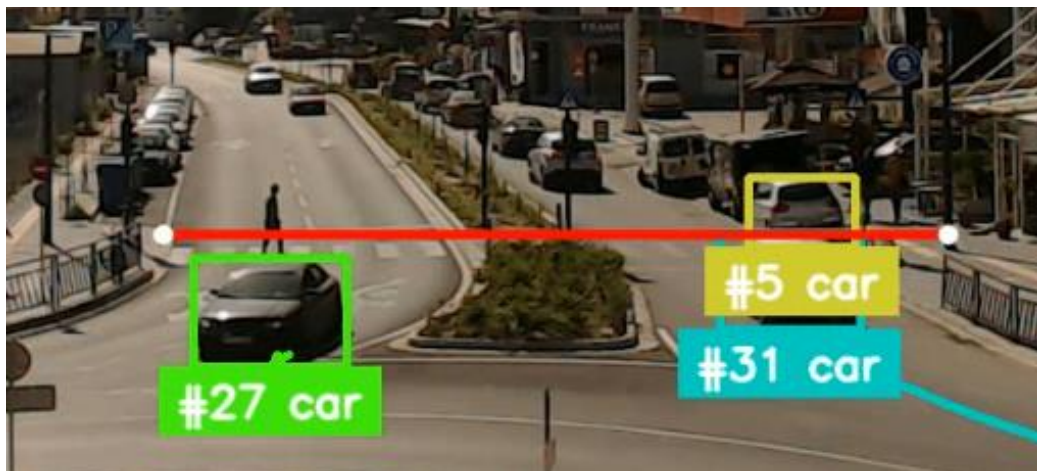
Figure 30: Virtual counting line
