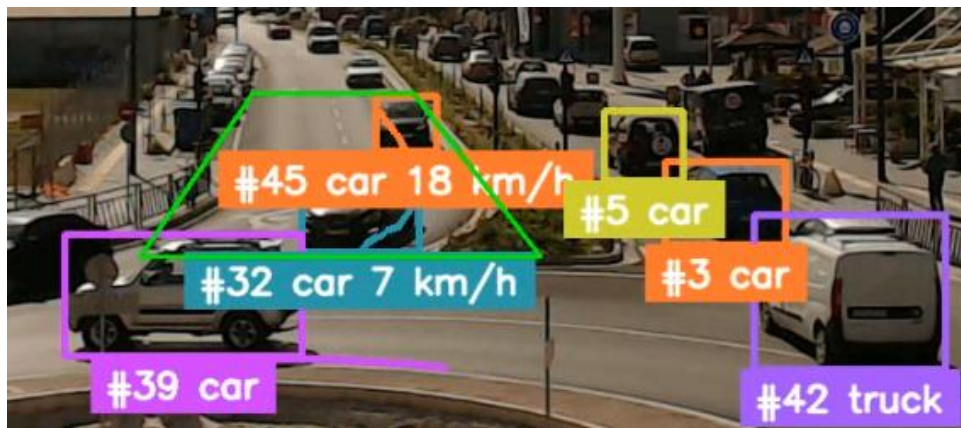
Figure 29: Speed estimation within SUBZONE
