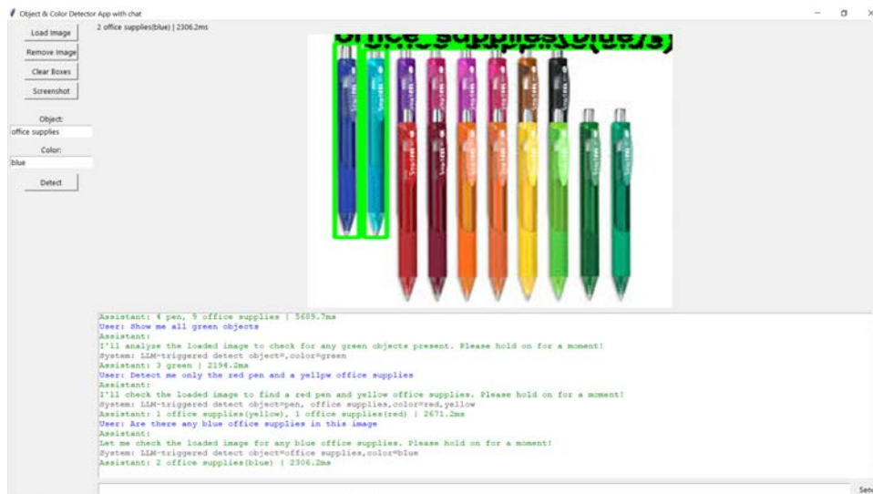
Figure 3.6: Detection of one specific colored object
