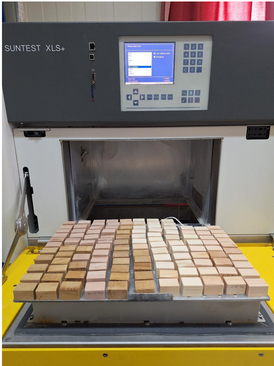
Photo 11: wood samples being placed in the xenon chamber
