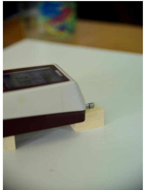
Photo 9: Surface roughness measured using the Mitutoyo SJ-210 roughness tester
