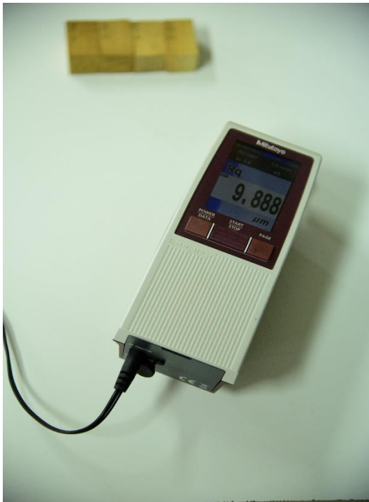
Photo 9: Surface roughness measured using the Mitutoyo SJ-210 roughness tester
