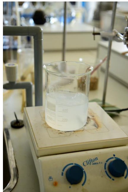
Photo 2: Silica nanoparticle solution in ethanol stirred on a magnetic stirrer for homogeneous dispersion
