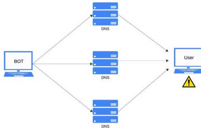
Figure 2.4: DNS amplification attack
