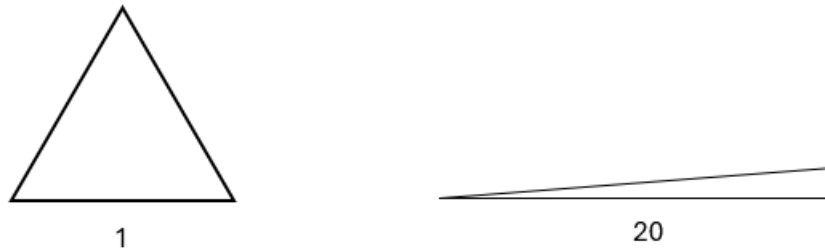
Figure 14: Depiction of aspect ratio on a triangular shape
