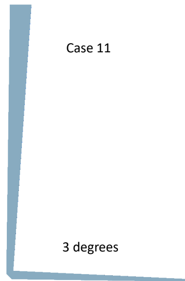
Figure 42: 3 degrees chimney wall angle
