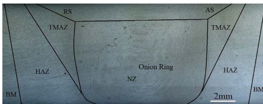
Figure 23 Macrostructure of FS weld [3]
