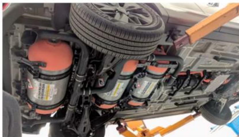
Figure 38. Hyundai Nexo 2019 with 3 small hydrogen tanks.
