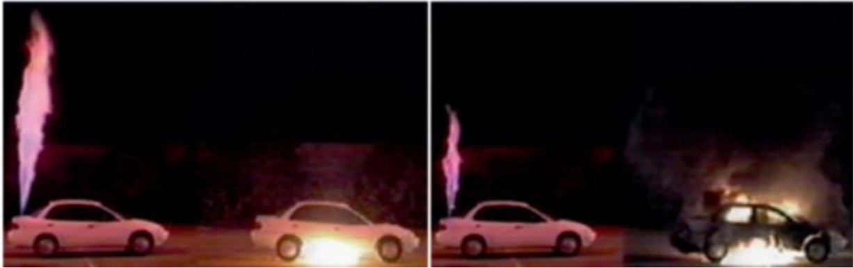
Figure 26. Generated fire by hydrogen and gasoline fuel at 3 s (left) and 60 s (right).
