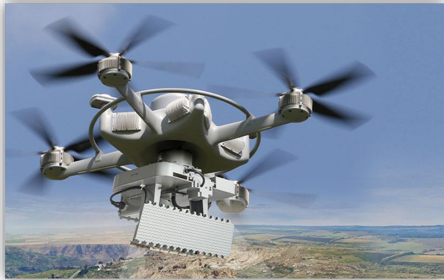
Figure 4: IAI ELTA's ELM-2054 Synthetic Aperture Radar UAV mounted (Source: [261])
