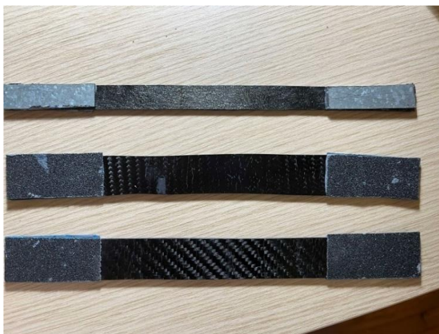
Figure 2.1 The upper specimen is made of Unidirectional Fabric and the other two are made of Bidirectional Fabric
