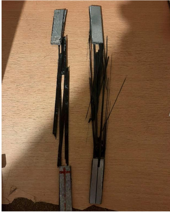
Figure 2.20 Failure mode at 0° orientation
