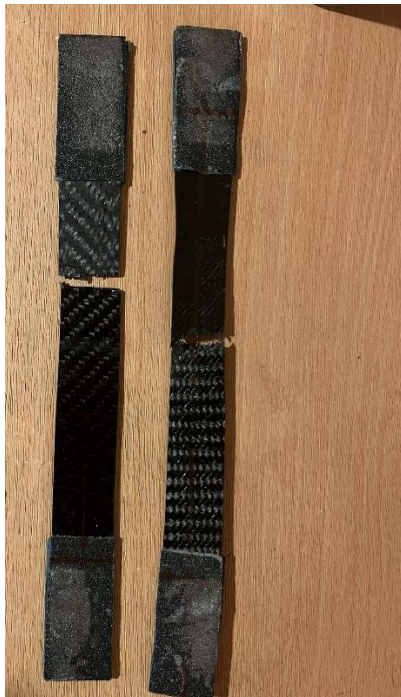
Figure 2.21 Failure mode at 0°| 90° and -45°|45° orientations
