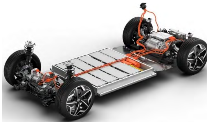
Figure 2.1: A typical BEV battery stack [55].
