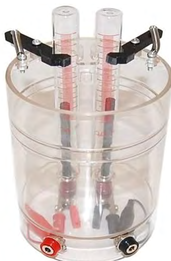
Figure 2.2: An electrolysis device [61].
