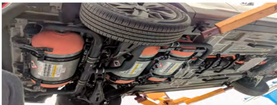
Figure 4.8: Fuel tanks of a Hyundai Nexo [51]
