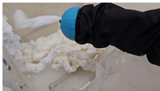
Figure 2.3: Hybrid robot showcasing adaptability in simulating Scenario 3, employing an expanding foam application to effectively cover the walls of the glove box. [1]
