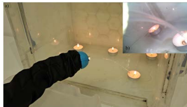
Figure 2.2: a) Hybrid robot demonstrating its versatility in simulating effectively extinguishing a candle's fire by employing a water-spraying mechanism. b) A POV view of the target, using the built in tip mounted micro camera [1].
