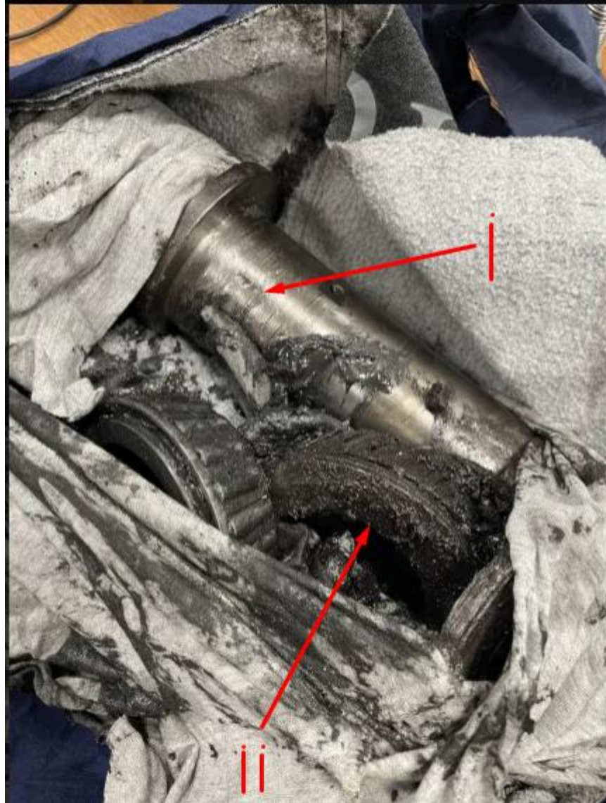
Figure 2.7: i) Cracks on the surface of a failed used shaft and ii) cracks which led to the total catastrophic failure of the big sized ball bearing.
