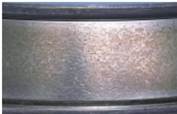
Figure 3.2: Brinelling observed on the inner ring raceway surface of the bearing.
