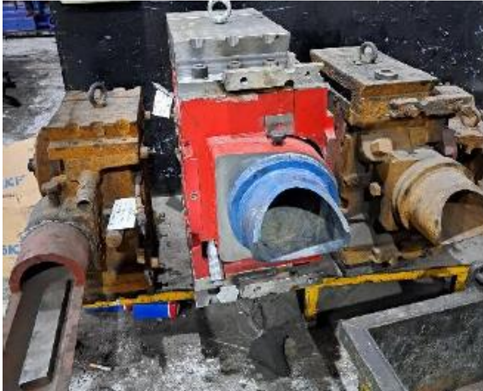
Figure 2.2: Front view of various twist exit roller guides from the maintenance workshop.
