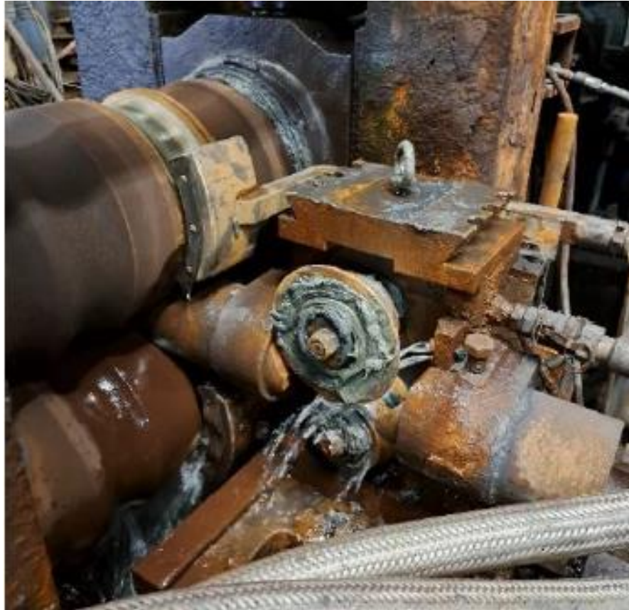
Figure 2.4: Twist exit roller guide assembled on the rolling cylinders just before a production cycle starts.
