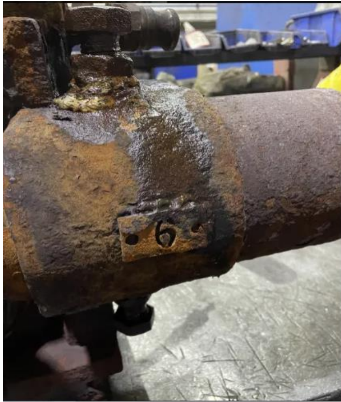
Figure 4.1: Wear observed on the outer surface of the twist exit roller guides.
