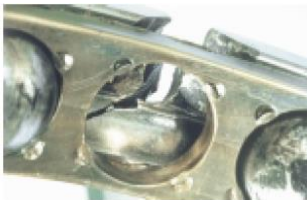
Figure 3.3: Crack detected on the outer ring of the bearing.
