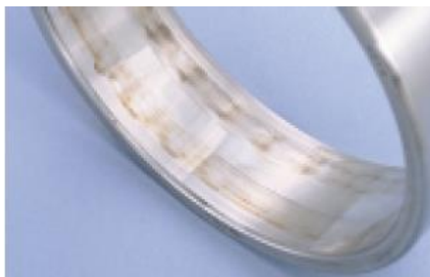
Figure 3.4: Scratch identified on the outer ring raceway surface of the bearing.
