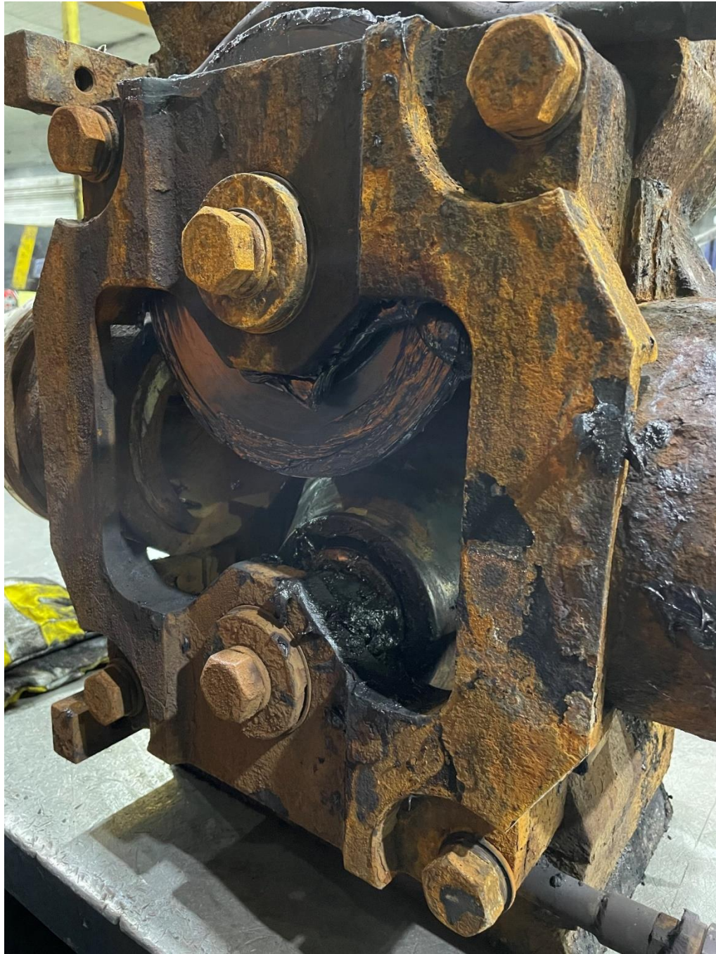
Figure 2.1: Side view of a twist exit roller guide after a production cycle.
