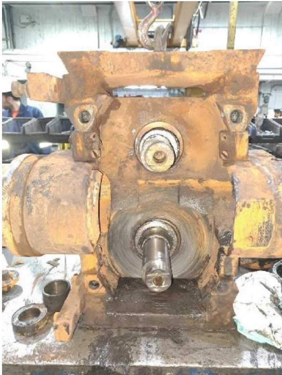
Figure 2.6: The wear observed on the body surface, resulting from contact with the lower roller, can be attributed to the substantial accumulation of grease and chips on the base surface.
