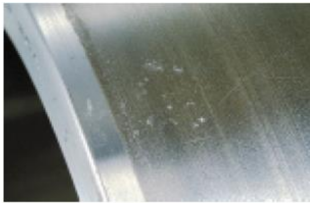
Figure 3.1: Pitting on the inner ring of the bearing.
