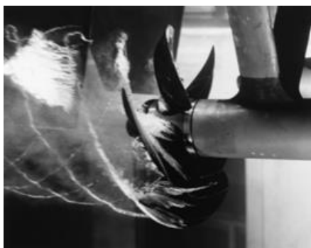
Figure 2. 7 Bubbles formed at the edges of the propeller, where the velocity is highest.
