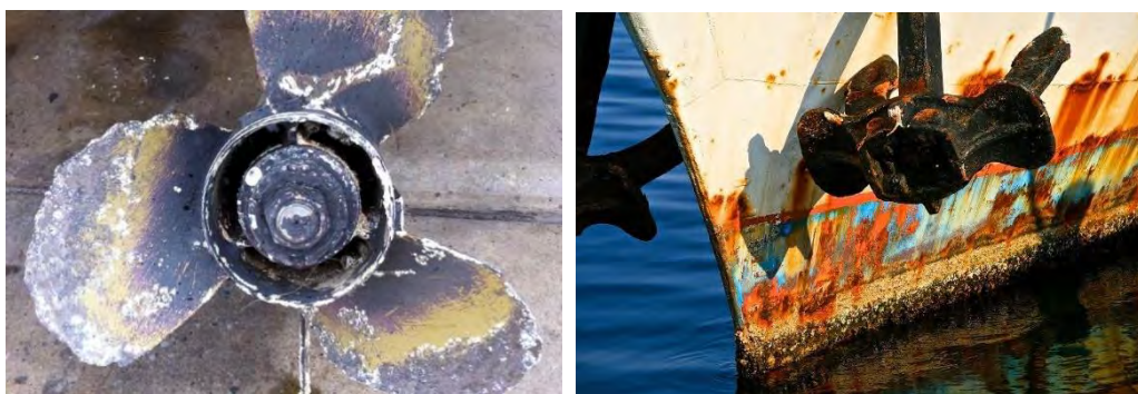
Figure 3. 30 (a) Galvanic corrosion on ship propeller, (b) Galvanic corrosion caused by metallic paint
