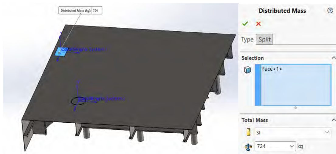
Figure 5.18 Weight distribution on the deck-mounted chock
