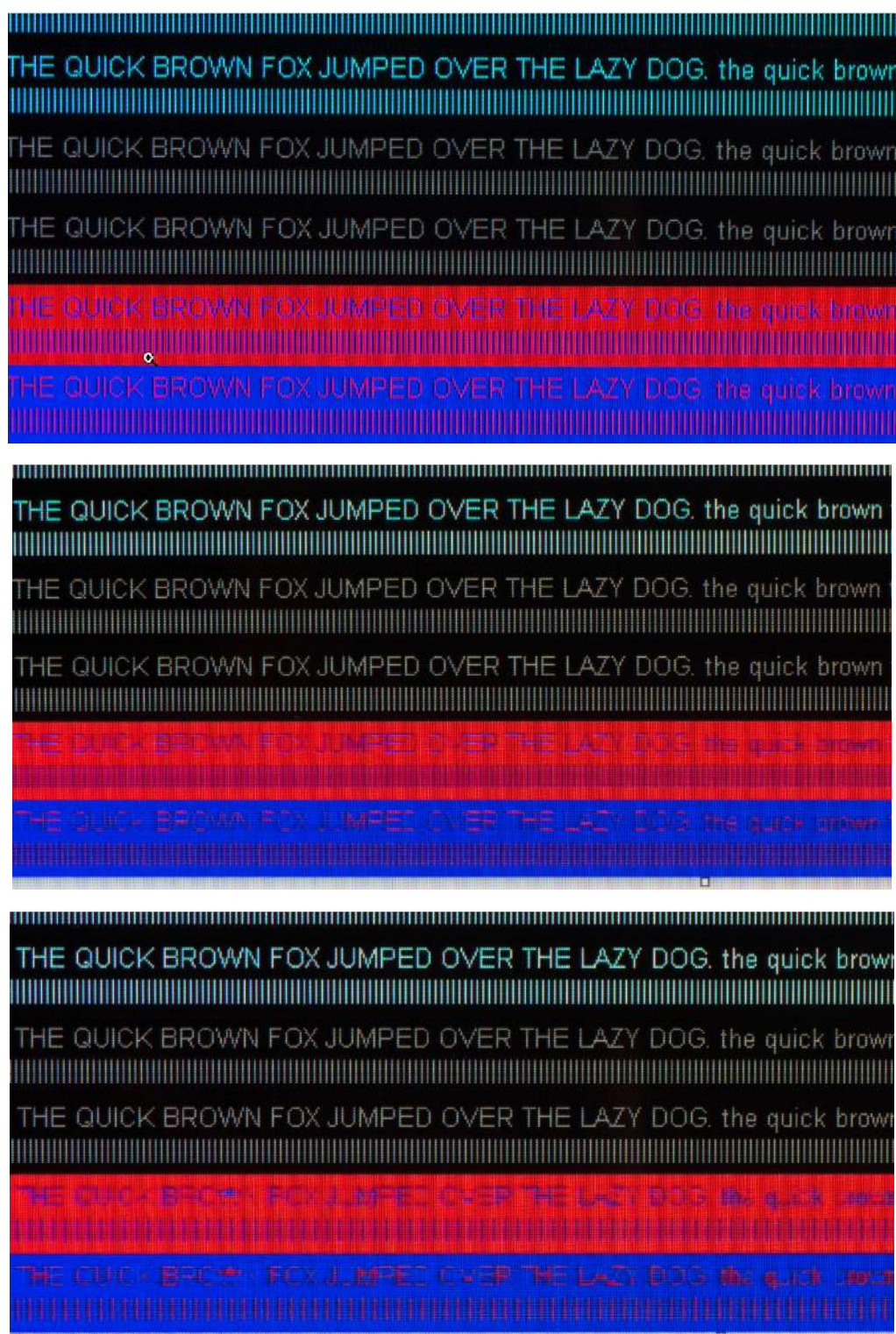
Figure 2. Chroma subsampling comparison. From top to bottom (a) 4:4:4 (b) 4:2:2 (c) 4:2:0
