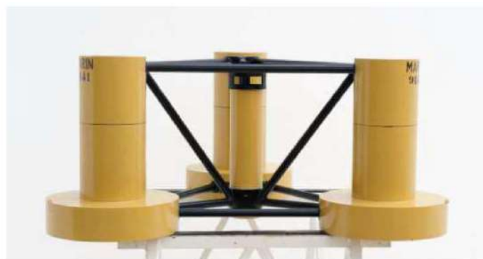
Figure 32: DeepCwind semisubmersible OC4 platform (as-built)[47].
