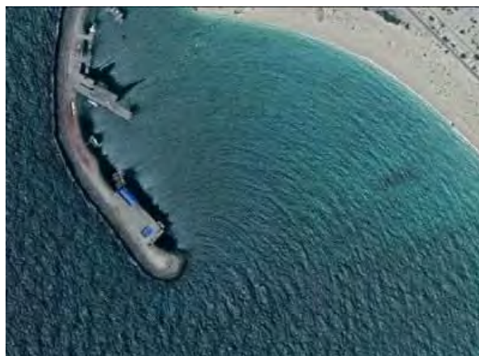
Figure 6: Diffraction of waves around the tip of a breakwater [16]
