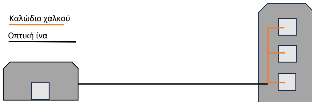
Σχήμα 2.23 Fiber To The Building
