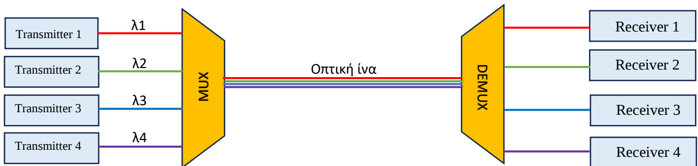
Σχήμα 1.3 Wavelength Division Multiplexing (WDM)
