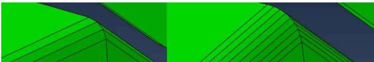
Figure 2.2.5: Automatically and manually segmented fillet
