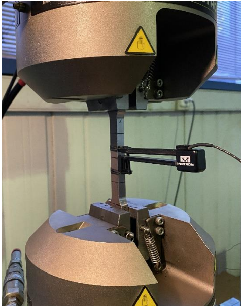
Figure 26. Extensometer on the coupon with rubber bands.
