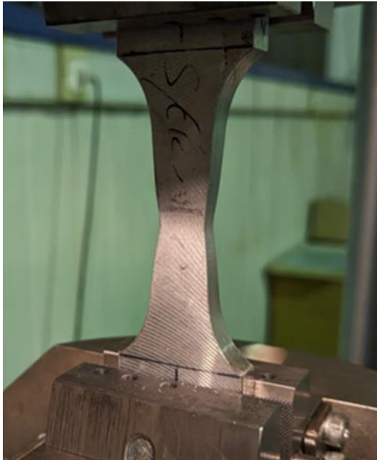
Figure 55. S355 Necking under stress control fatigue
