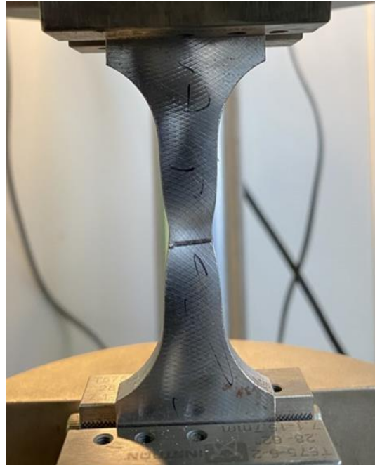
Figure 56. S700 necking under stress control fatigue
