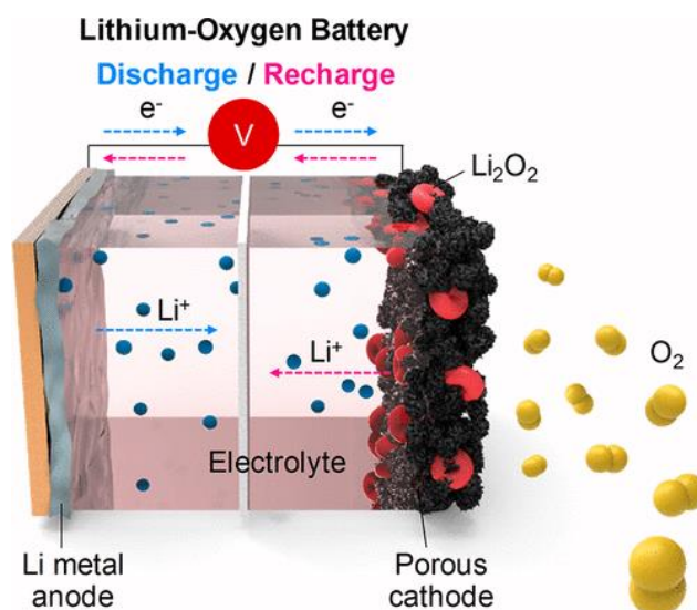
Figure 2.7: Schematic presentation of \text{Li-O}_2 battery [37]
