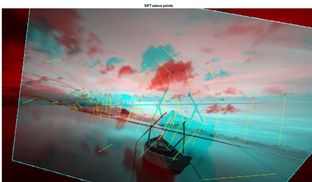
Figure 4. The image pair presented in Figure 3 was analyzed and warped as instructed in chapter 0 using the SIFT feature extraction method and warped the moving image to match the fixed one.
