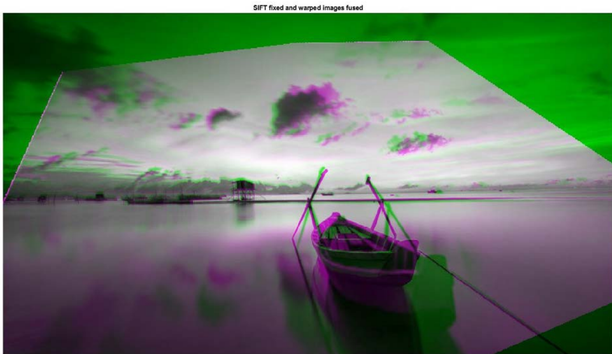
Figure 5. After finding the feature points through SIFT, the projection transformation matrix is estimated based on those points. The moving image is warped and fused with the fixed one to make results easier to the eye.
