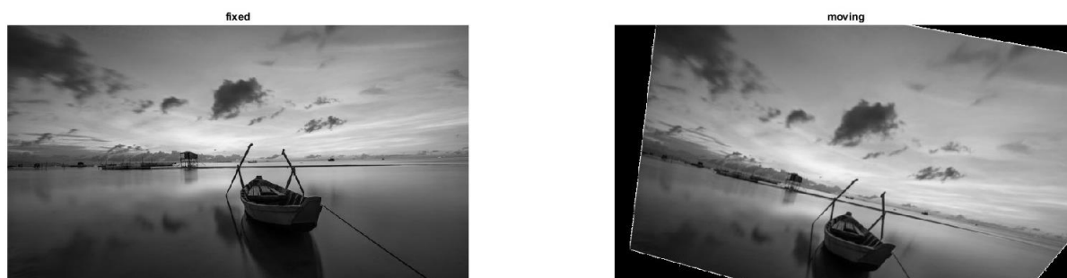
Figure 3. A random image showing a boat was warped with a random Homogeneous transformation. The original image (fixed) is on the left and the randomly transformed image (moving) is on the right.
