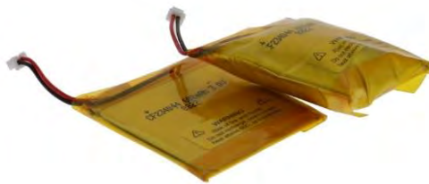
Figure 25 : In the picture it is depicted the same pouch cell but on the right side it is swelled significantly [17].
