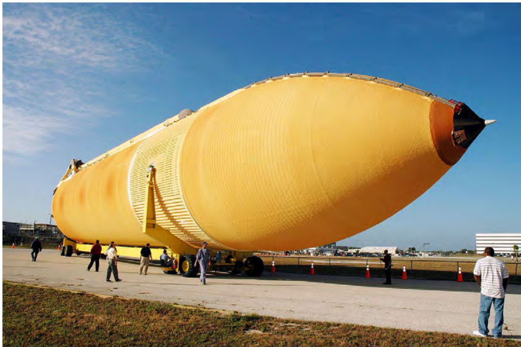
Fig. 5: Tank construction by NASA using Al-Li alloy, SLWT [15]
