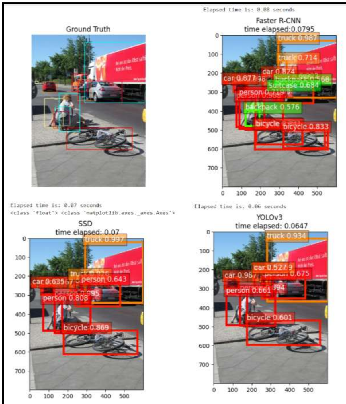
Fig 3.2. The results of SSD, YOLOv3, and Faster R-CNN tests.
