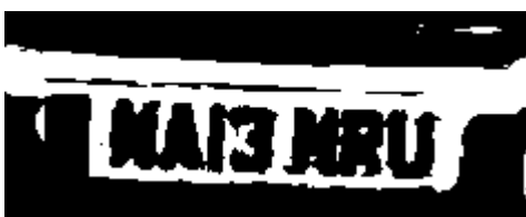
Fig 3.3.5 Bitwise not Thresholded Image.
