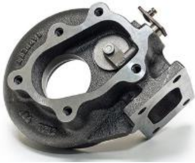
Figure 18 a. Internal wastegate [41]
