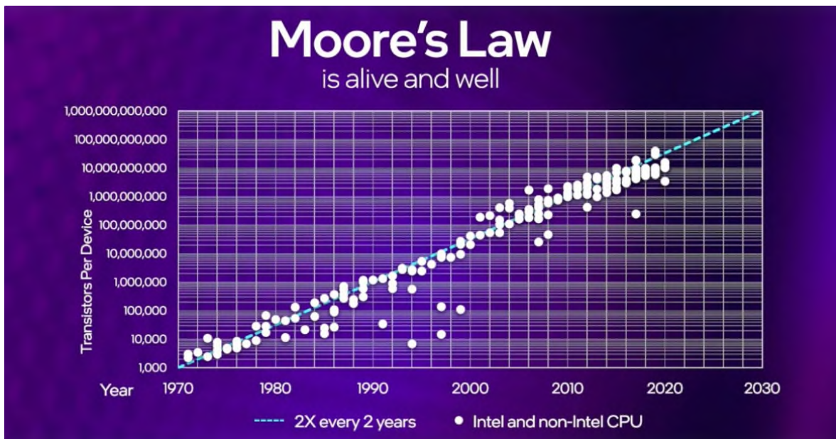
Figure 1.4: Presenting the number of transistors used in produced well-known chips from 70s until now, perfectly aligned with the prediction of Gordon Moore's law [21].
