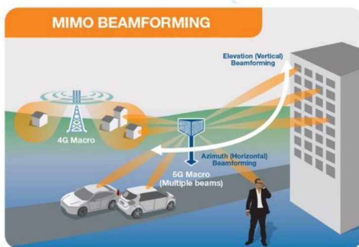
Figure 4.12. 4G VS 5G MIMO antenna with beamforming. 4G beam covers an area with many receivers while the beamformer directs dedicated beams to users. Source: ITU (Poland, 2017 conference).
