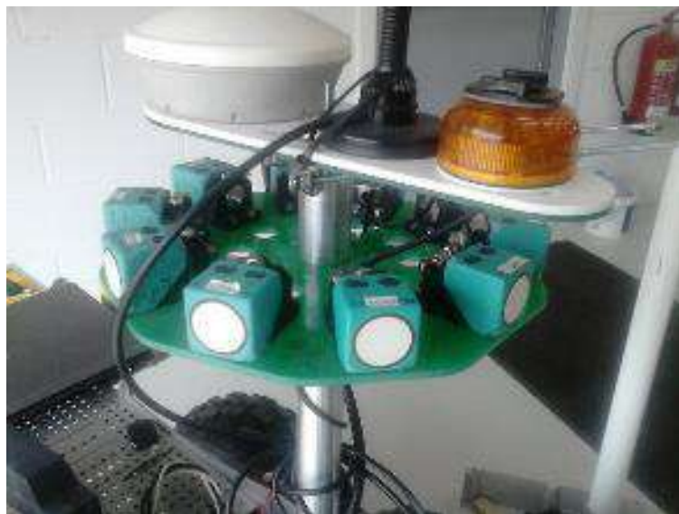
Figure 94: Ultrasonic system with 10 sensors
