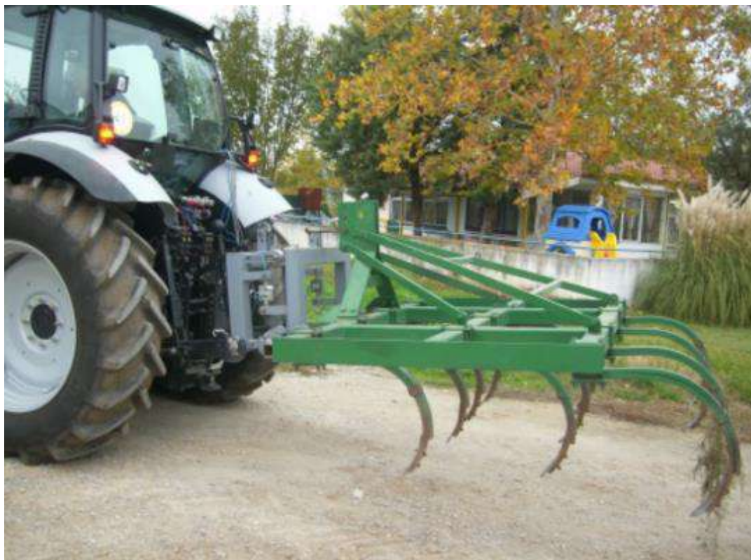
Figure 50: Duty rigid type cultivator attached at the three-point hitch dynamometer
