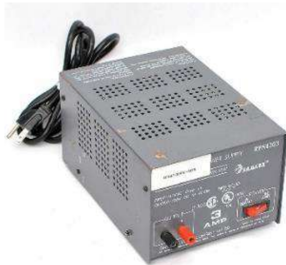
Figure 43: 13.8V regulated DC power supply
