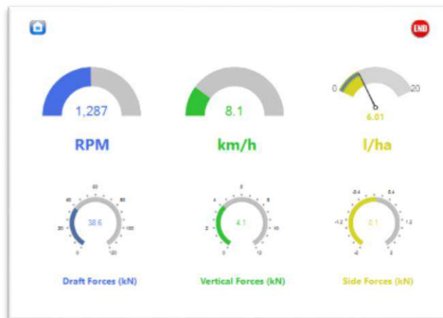
Figure 81: HUD (Head-Up Display) projecting values in real time
