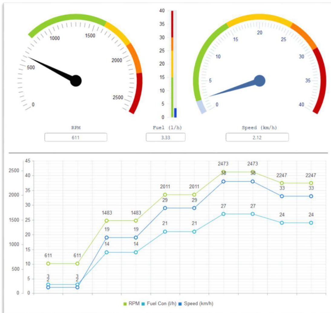
Figure 32: Real time data projection (telematics) from a tractor
