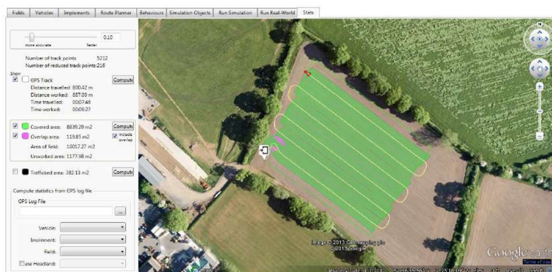
Figure 132: Route following and efficiency
