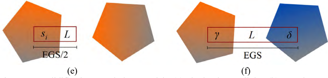
Figure 4.9. Solidification morphology models: (a) Single-phase cellular, (b) two-phase cellular, (c) single-phase dendritic, (d) two-phase dendritic, (e) single-phase equiaxed and (f) two-phase equiaxed.
