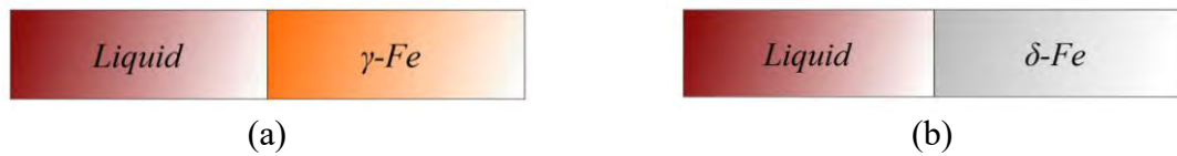
Figure 4.5. Single-phase solidification cells: (a) Single austenite AL for type-A and (b) single \delta -ferrite FL for type-F.
