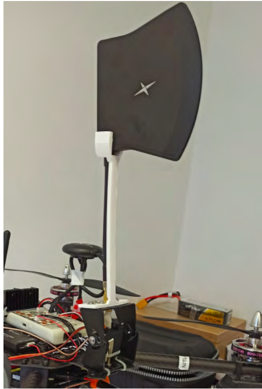
Figure 2.13: Directional Antenna mounted on a UAV
