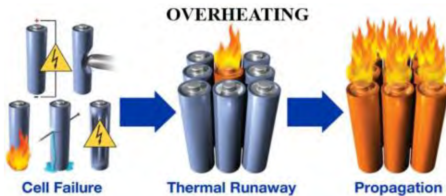
Figure 4.3. Thermal runaway effect on battery [317].
